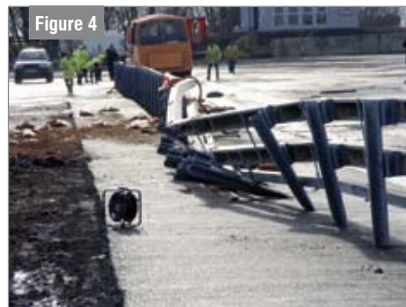
Figure 4 A deformable steel safety barrier following TB51 test
