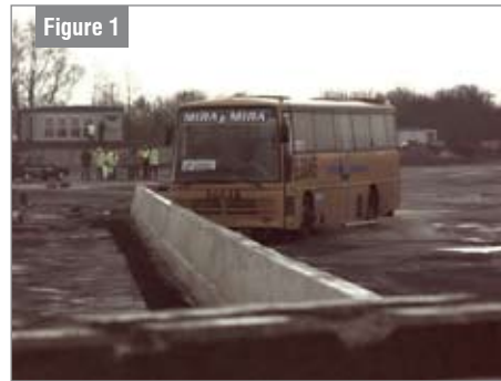
Figure 1 TB51 test showing 13t bus at 70kph approaching CSB at 20°
