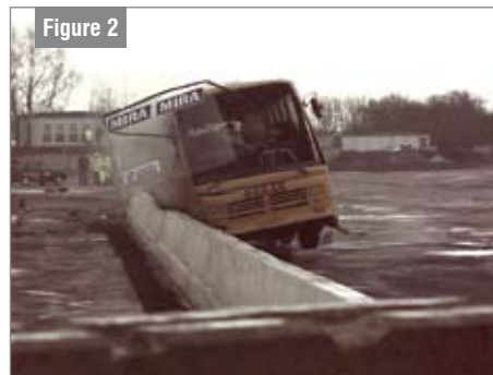
Figure 2 TB51 test showing 13t bus after impact with CSB
